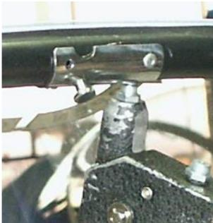
Position the supplied upper pin on the rear canopy frame and align it with the original holes through the frame. Rivet it with blind rivets 3.2x7.9 mm (4 pcs). Use a hand riveter.
