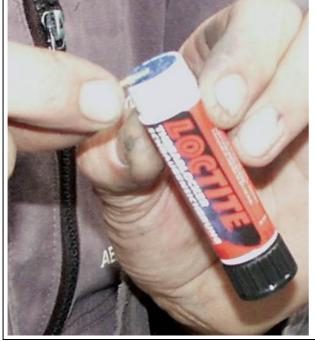
Apply small amount of Loctite threadlocker (e.g. 243 or 245) on the M3 screw threads.
