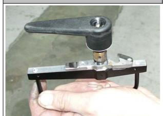
Put the locking hook on the new handrail. Slip the pivot of the handle into the hole in the locking hook and handrail body to set position of the locking hook on new handrail.
