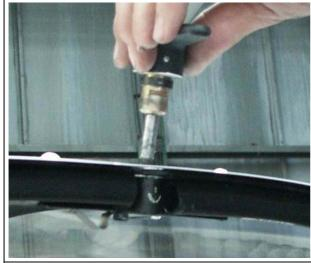
Pull the handle with pivot upwards out of the canopy frame.
