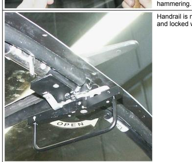
Handrail is now assembled with the handle pivot and locked with the pin.
