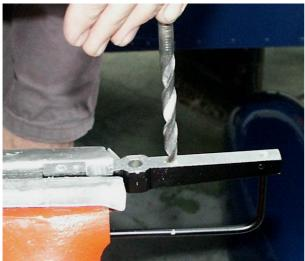
Countersink the holes with a bigger diameter drill
