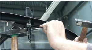
Use ejecting pin  $\varnothing$  2.8 mm to eject pin  $\varnothing$  3 mm from handle pivot.
