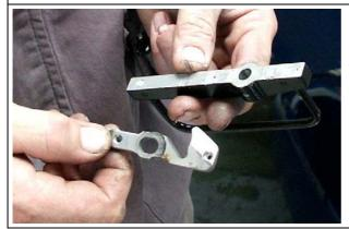
Remove locking hook from the original handrail.
