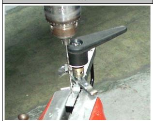
Turn the locking hook slightly and drill the hole through whole handrail body.
