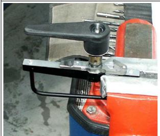
Chuck the handrail with handle in a vice.
