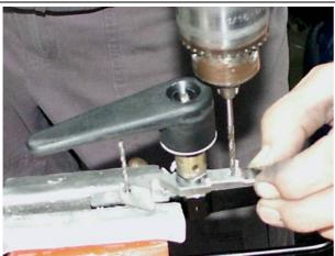
Use a drill bit or wire of suitable diameter to align locking hook hole with the drilled hole.
