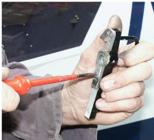
Unscrew two M3 screws attaching locking hook to the original handrail.
